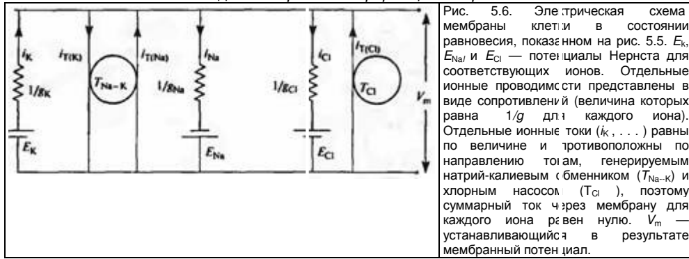
Fig. 5.6. Electrical Model of the Steady-State Cell Membrane shown in Figure 5.5. E_K , E_{Na} , and E_{Cl} are the Nernst potentials for the individual ions. The individual ion conductances are represented by resistors (having a resistance of 1/g for each ion). The individual ion currents ( i_K , i_{Na} , and i_{Cl} ) are equal and opposite to the currents ( i_{T(K)} , i_{T(Na)} and i_{T(Cl)} ) supplied by the sodium-potassium exchange pump ( T_{Na-K} ), and the chloride pump ( T_{Cl} ), so the net flux of each ion across the membrane is zero. The resulting membrane potential is V_m .
