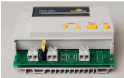
Fig. 1. Battery charge controller.
