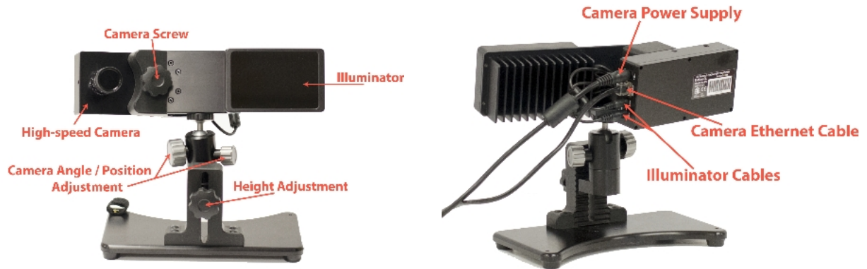
Figure 3-2: Parts of the EyeLink 1000 Plus Desktop Mount
