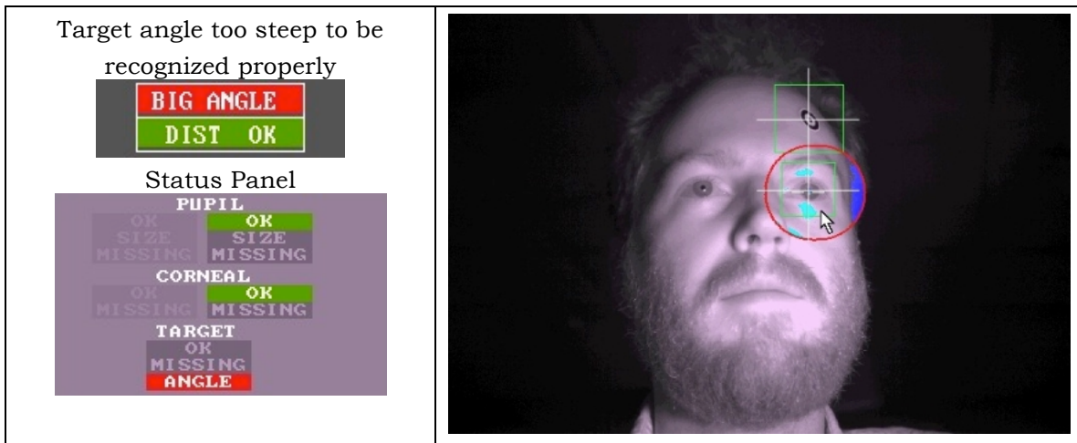
Figure 3-7: EyeLink Remote Target Placement
