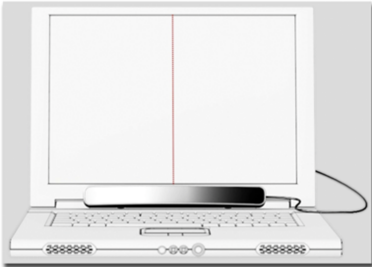
Device centered and resting in hinge area of Laptop
