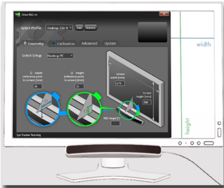
Measuring screen height and width
