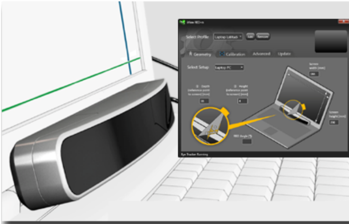
Measuring width and height of screen
