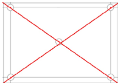
Wrong 5-point calibration scheme
