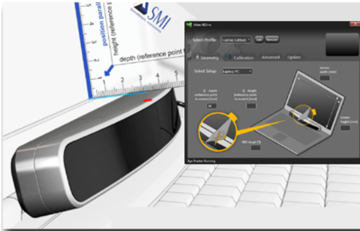
Measuring depth offset
