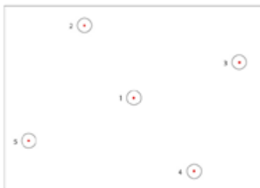
Correct 5-point calibration scheme
