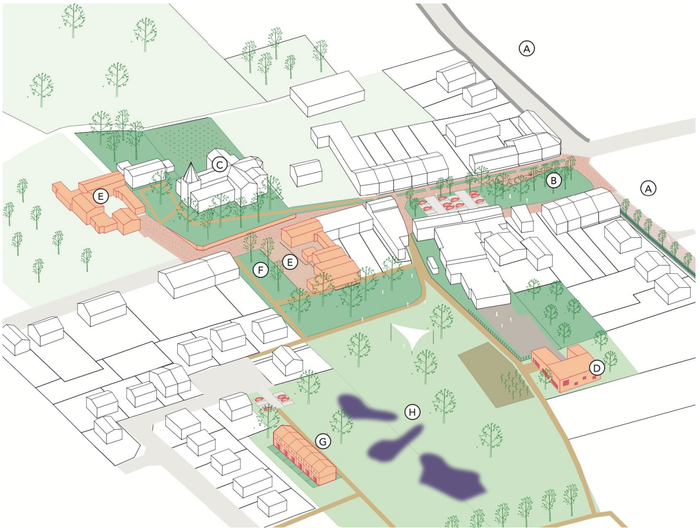
fig. 4. Design research for the village of Neerlinden looking at alternative profiles for the main street (a), de-sealing operation on the village square (b), the reuse of the vacant church building (c), the position of the school extension (d) and new pedestrian passage (f) in relation to the shared gardens and waterpark (h) with additional housing (g), and the reuse of remarkable abandoned farmhouses (e). (by Plusoffice Architects, Leefbare Dorpen Getestreek, 2020).
